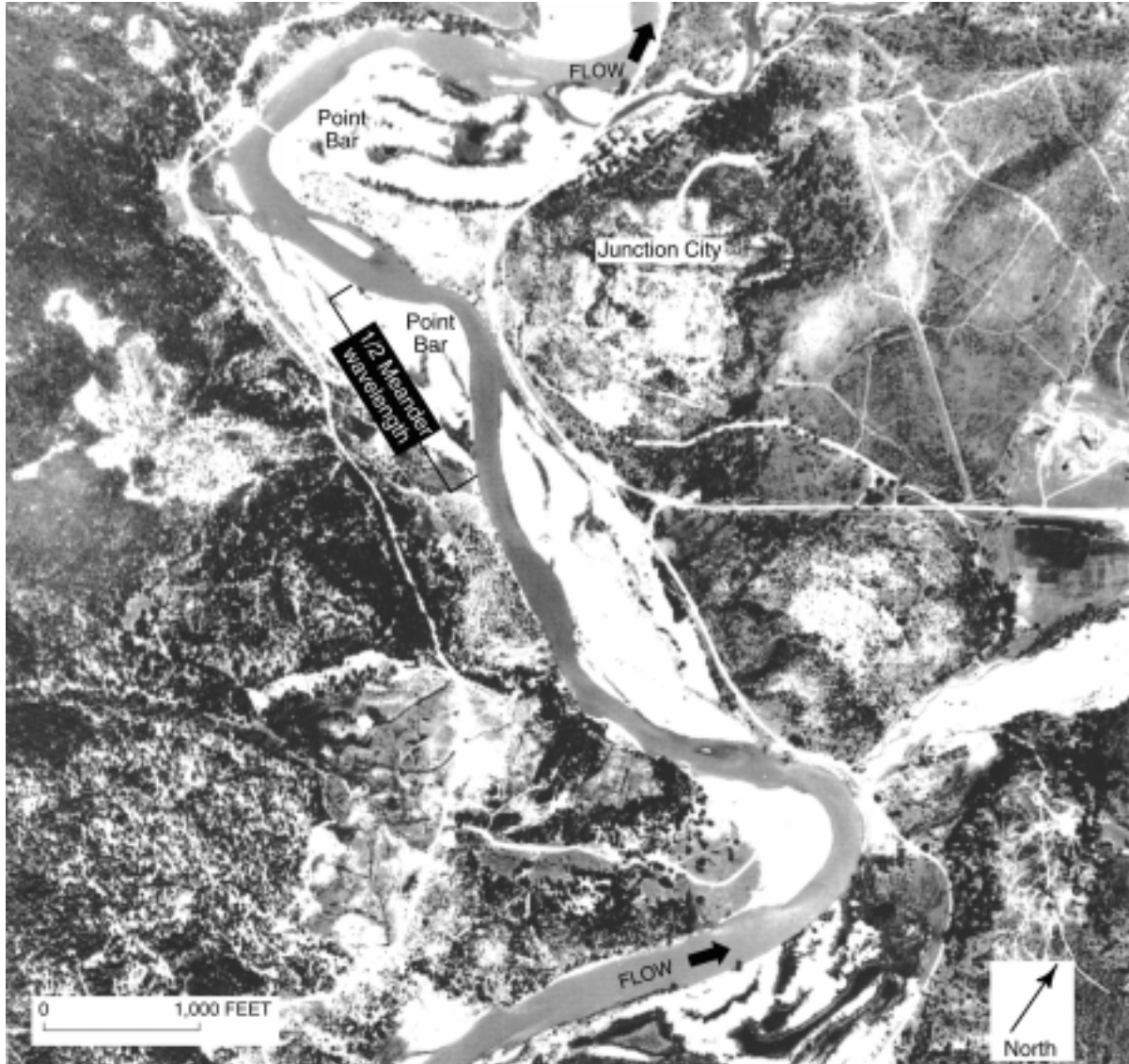
Figure 4.3. Trinity River at Junction City (RM 79.6) in 1960 illustrating alternate point bar sequences at a discharge of 5,000 cfs.
