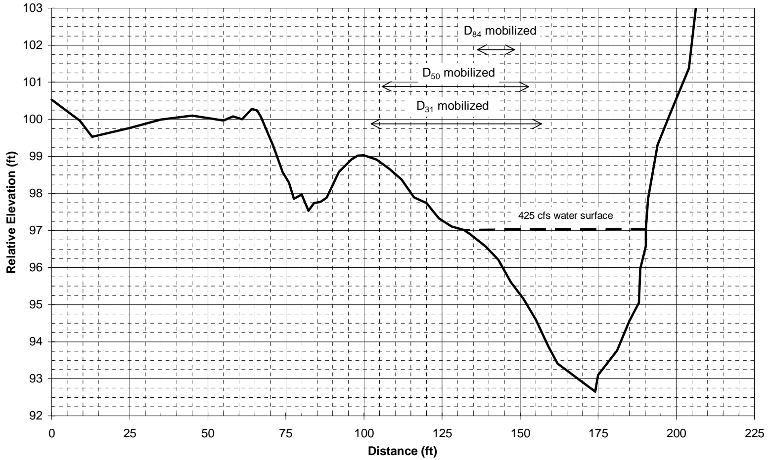
Figure 5.30. Bed mobility pattern at Bucktail bank-rehabilitation site (RM 105.6), cross section 12+00 during 5,400 cfs release. Rocks placed from station 96-156.
