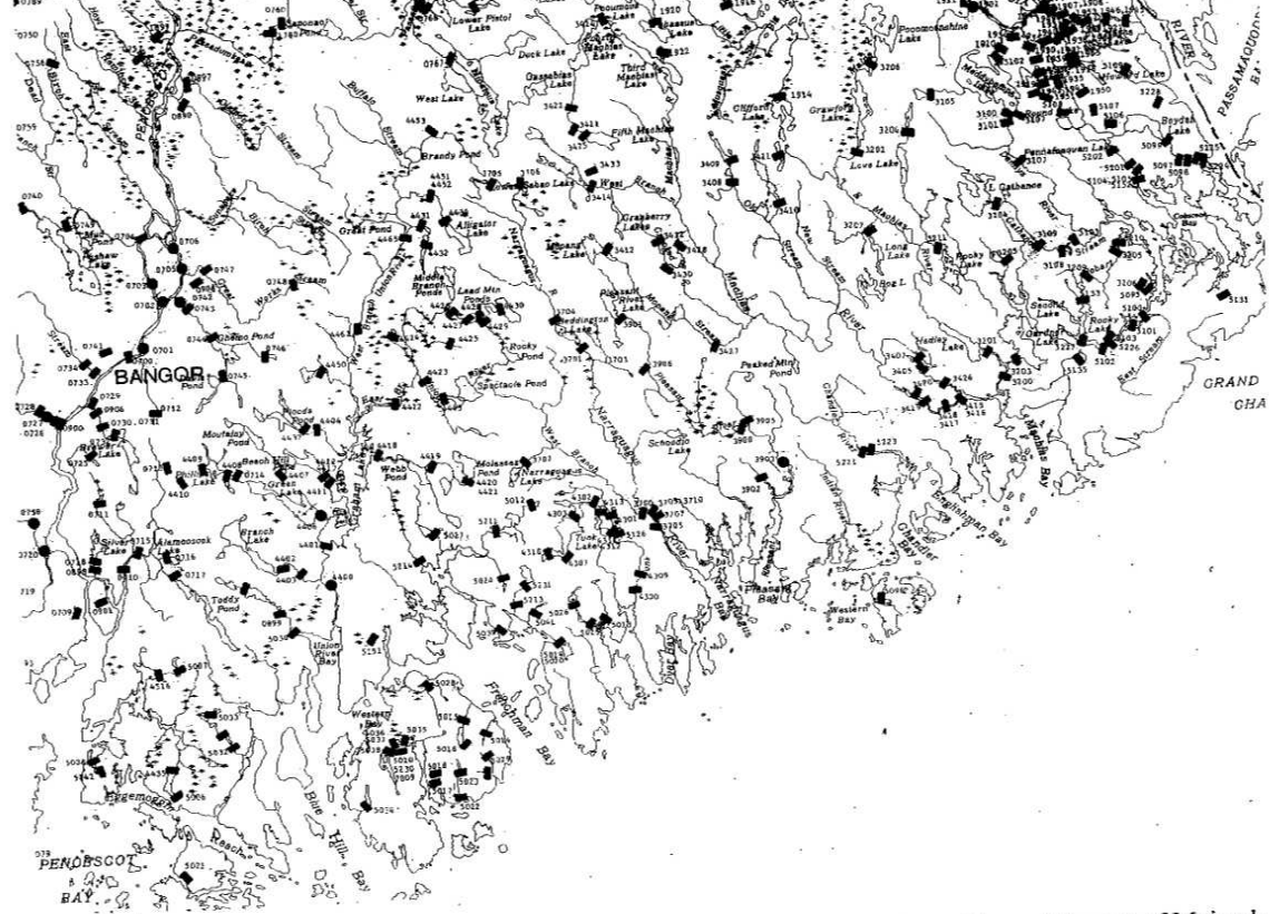
FIGURE 3-2 Existing and former dams in Down East Maine, including part of the Penobscot River. The rest of Maine looks similar. A black rectangle indicates one non-generating dam, and a black circle indicates one hydroelectric/power dam. The numeral beside each dam site corresponds with data provided in the Inventory of Existing and Former Dams in Maine (Elder 1987). Source: Elder 1987.
