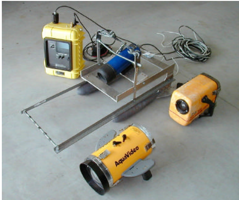
Figure 7. Three underwater camera systems used by the author to record underwater observations of fish and habitats in rivers. Camera at top center is configured for riverbed substrate surveys. The system is described in the report. Two 30-lb. streamlined weights hold and orient the camera in very fast water. Cameras at bottom and right are self-contained units for use by SCUBA divers.
