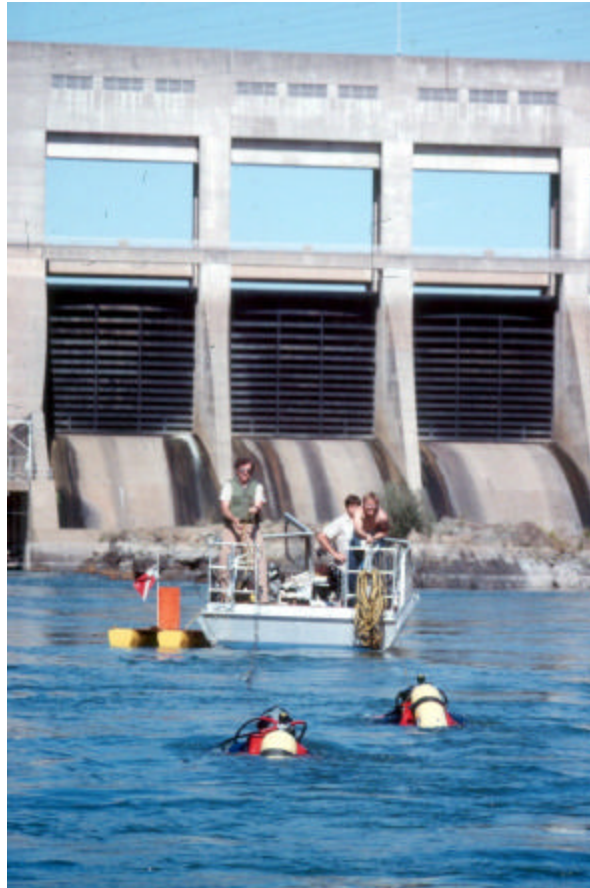
Figure 6. SCUBA divers preparing for riverbed surveys immediately downstream of Keswick Dam on the Sacramento River in water depths up to 40 feet. Author (SCUBA diver in left foreground) is “hard-wired” to the jet boat with a tow line and underwater communications cable. The two divers used planing boards to descend to and ascend from the riverbed in the fast currents.
