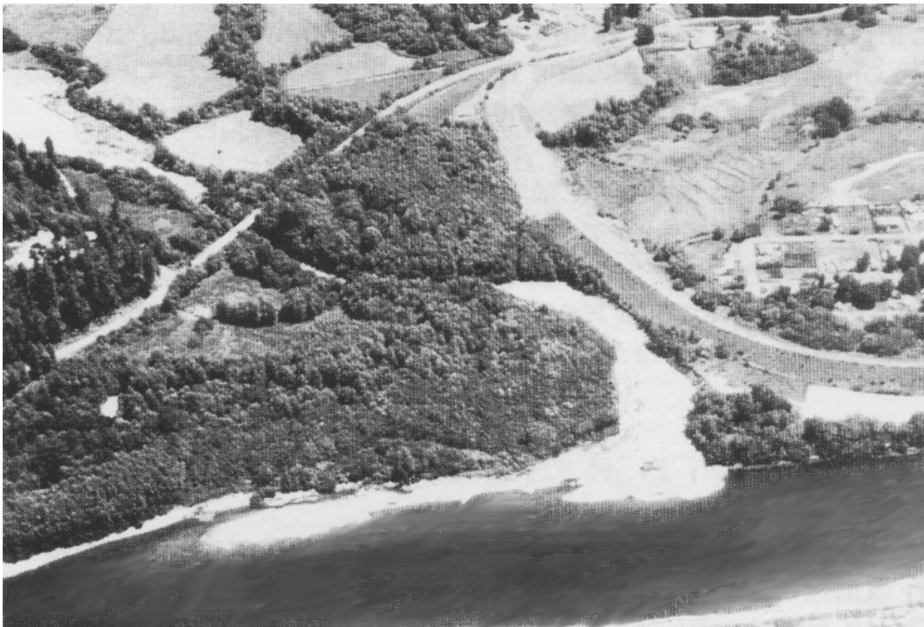
Figure 3-7 -- Turwar Creek runs underground at its confluence with the Klamath River because of its tremendous sediment load. The Klamath has also been filled in by sediment transported from throughout the watershed.
